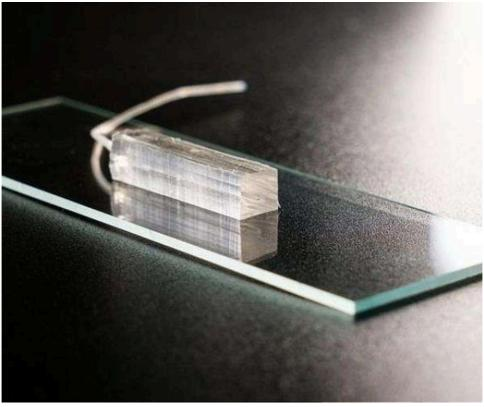
Close-up of the microfluidics device which can make square-shaped micro-ceramic particles with sharp corners.
